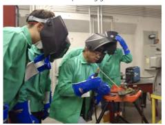
BM Val Ceria demonstrating a lap joint on two pieces of steel plates.
